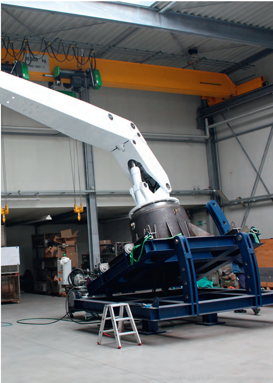
Deck crane for rescue boat
